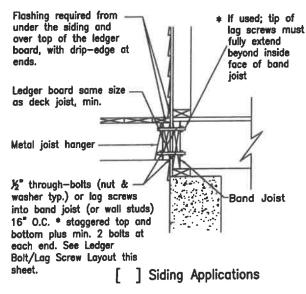
½" through-bolts (nut & washer typ.) or lag screws into band joist (or wall studs) 32" o.c. staggered top and bottom plus min. two bolts at each end. Additional support using Option 1 or 2 (or approved equivalent) must also be provided. See Layout this sheet.
